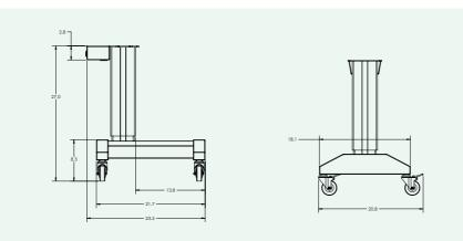
Table height dimensions with table top included: Lowest position to floor: 28" (71cm) Highest position from floor 35.75" (91cm) Total lift measurement 7.75" (19.5cm)
