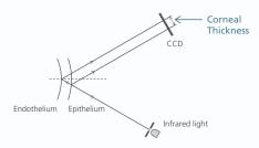
The principle of specular reflection for pachymetry allows a more compact design of TONOREF™ III.
