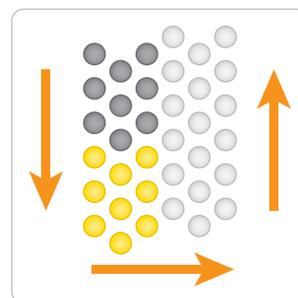
The repeat mode with the auto forward function enables consecutive regions to undergo photocoagulation on a selected path without repeatedly pressing the foot switch.
