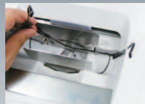
Composite tracing measures the FPD/DBL and frame wrap angle along with the frame shape, thus, calculating all frame measurements automatically.
