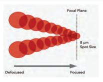
YAG twin aiming focusing system allows both beams to converge together at the focal target to create a sharp and precise spot.
