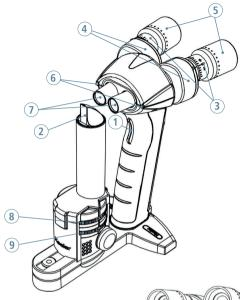
Magnification change lever (PSL Classic only): Push this lever to the right to set the magnification at 10x and to the left to set the magnification at 16x.
