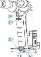
14. Brightness adjustment wheel: Rotating this wheel clockwise increases the brightness of the illumination lamp. Rotating this wheel anti-clockwise decreases the brightness of the illumination lamp.
